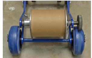
Liner take-up bar is fully installed.
