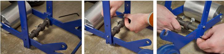
Align the parts (left), insert the hex screws from the inside (center), and add the nuts from the outside (right).
