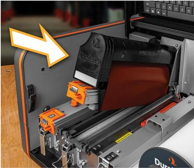
3. Slide the cartridge onto the rails of the print head. It should slide smoothly back until the number on the print head is visible; you may hear the cartridge click into place.
