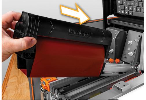
2. Holding the ribbon cartridge on the side imprinted with the DuraLabel logo (with the rolls facing up), insert it into the printer so the loose section of ribbon, on the bottom side of the ribbon cartridge, is positioned beneath the print head.
