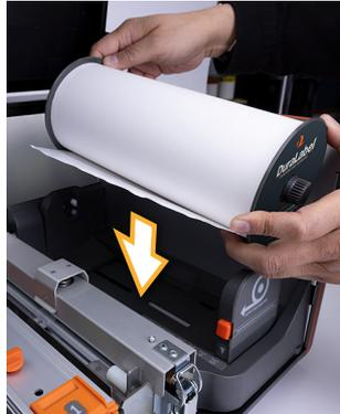
2. Rest the gears on the supply's end caps into the slots on the supply holders. The end cap with the DuraLabel Printers and Supplies label should face away from the inner wall of the printer.
