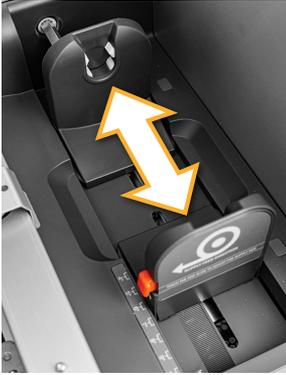
1. Squeeze the orange tab on the adjustable supply holder, and slide the holder to the mark for your supply's width.
