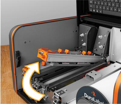
1. Unlatch one of the print heads and raise it by its orange tab until it can no longer be raised where it will hold.
